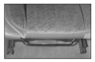
If your vehicle has manual seats, lift the bar located under the front of the seat to unlock it. Slide the seat to where you want it and release the bar. Try to move the seat back and forth to be sure the seat is locked in place.
